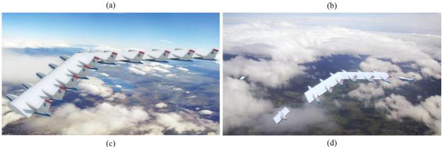
Figure 2. Conceptual image of the Cluster Wing vehicles (a) Takeoff with tow aircraft (b) Tow aircraft releases the Cluster Wing at top of climb (c) Vehicles together during cruise (d) Vehicles separating to complete mission
