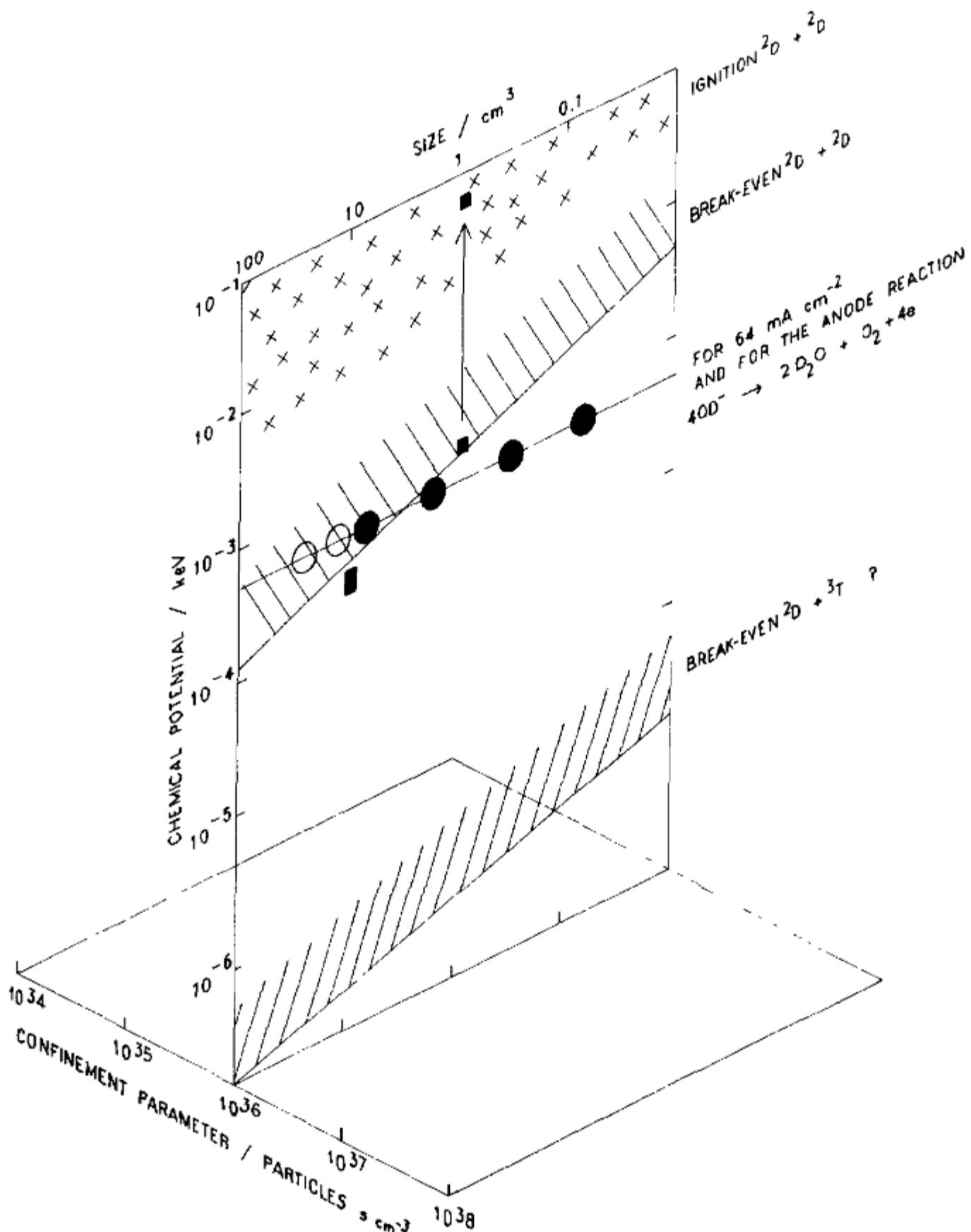
Fig. 2. Confinement parameter-chemical potential-size diagram for  ${}^2\text{D} + {}^2\text{D}$  fusion reaction in Pd cathodes; projection to the  ${}^2\text{D} + {}^3\text{T}$  reaction. Open circles: systems currently being investigated.
